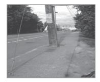
When utility poles are installed directly in the walkway, it can make wheel chair access a challenge, and further diminish the space allocated to pedestrians. Here, the worn area to the right of the sidewalk shows that pedestrians use this space in larger numbers than the sidewalk accommodates. Worn areas like this, or 'goat paths' across grass, are sometimes referred to as desire lines, showing the route that pedestrians desire to travel despite shortcomings in the built environment.
